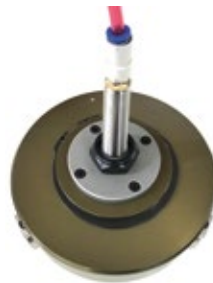
Example of chuck back side with MK2 shaft and rotary feedthrough
